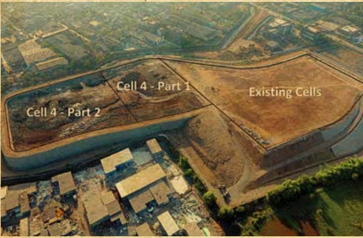
As mentioned above, the landfill is divided into cells, and each cell is filled one at a time. The first three cells were closed and covered as per statutory requirements. Strata developed Cell 4. To achieve this, Strata successfully executed the following:
